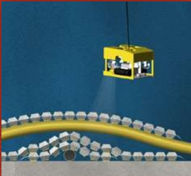
GROUT BAG INSTALLATION
